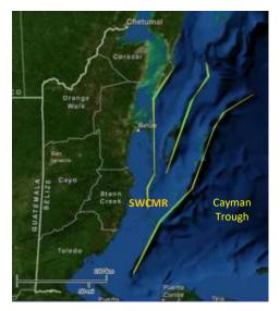
FIGURE 11: FAULT LINES / ESCARPMENTS RUNNING PARALLEL TO THE BELIZE COASTLINE, FORMING THE BASE OF THE BARRIER REEF AND ATOLLS (BASED ON PURDEY ET AL., 2003)
